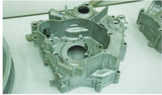
The company also handles die-casting molds for motorcycle.
