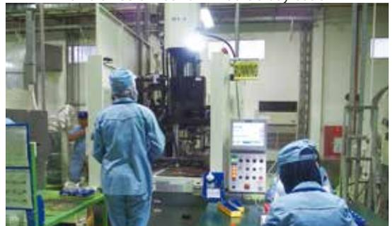
Insert molding machine running for mass production
